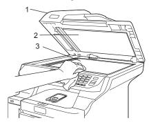
In the ADF unit, clean the white bar (1) and the scanner glass strip (2) underneath it with a soft lint-free cloth moistened with a non-flammable glass cleaner.
